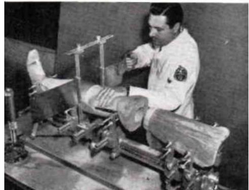
Fig. 23. Using the above-knee adjustable leg and alignment duplication jig. *Top*, adjusting the adjustable leg during walking trials; *center*, the socket and adjustable leg in the alignment duplication jig; *bottom*, replacement of the adjustable leg with a permanent knee and shank.
