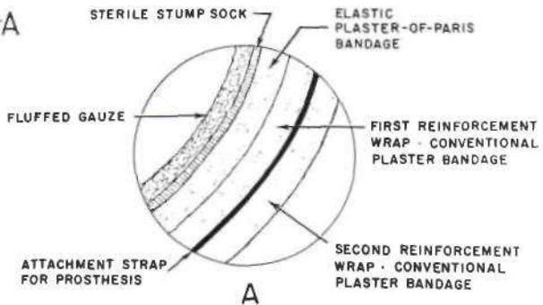
Fig. 18. Schematic cross section showing the major elements of a prosthesis as applied immediately following surgery to a below-knee amputee. The suture line, silk dressing, and drain are not shown. The fluffed gauze does not extend beyond the area indicated in "A." Inset: A below-knee amputee fitted with the immediate postsurgical prosthesis.
