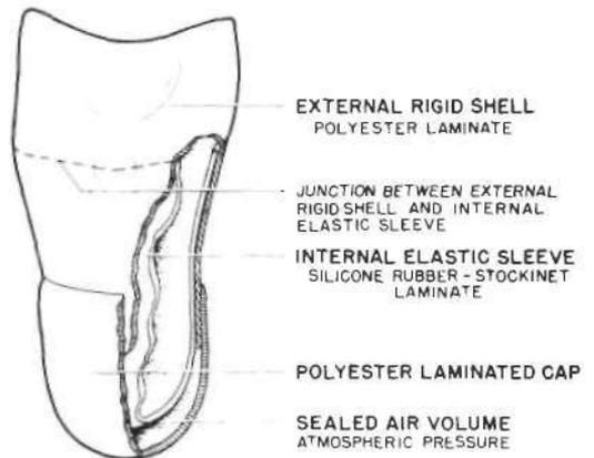
Fig. 34. Cutaway view of the air-cushion socket.
