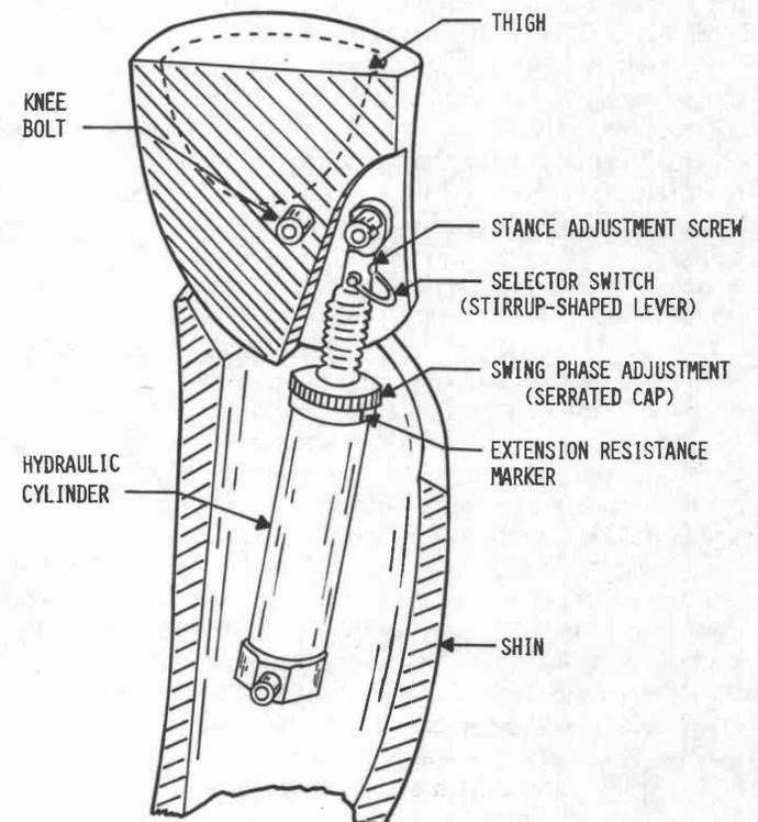
Figure 1. Cutaway diagram of the Mauch Unit
