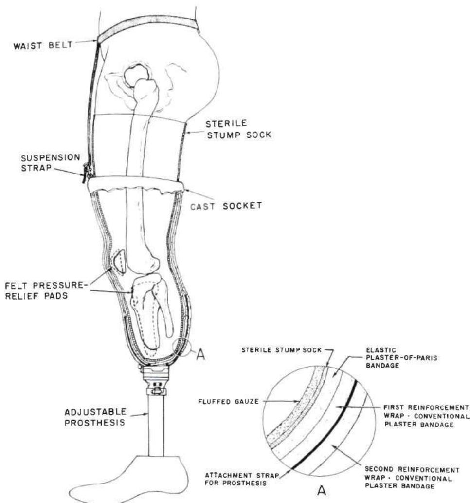
Fig. 18. Schematic cross section showing most of the elements of the application of a prosthesis to a below-knee amputee immediately after surgery. The suture line, silk dressing, and drain are not shown for the sake of clarity. View "A" is an enlarged schematic section of the cast socket, prosthetic unit attachment straps, stump sock, and fluffed gauze at the distal portion of the stump. The fluffed gauze does not extend beyond the area indicated.
