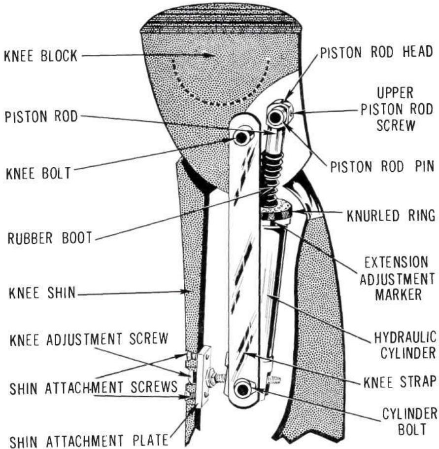
Fig. 33. The Henschke-Mauch "HYDRAULIK" set-up.
