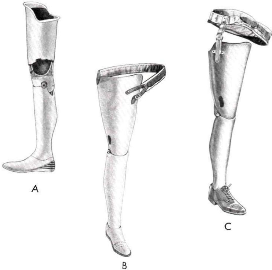
Fig. 36. Above-knee sockets and methods of suspension. *A*, Total-contact suction socket; *B*, above-knee leg with Silesian bandage for suspension; *C*, above-knee leg with pelvic belt for suspension. Most above-knee sockets have a quadrilateral-shaped upper portion as shown.
