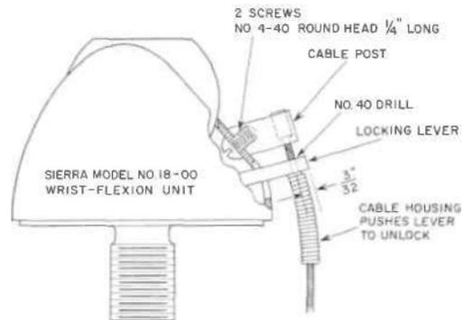
Fig. 4. Modifications of wrist-flexion unit for use with nudge control. Refer to Figure 1.
