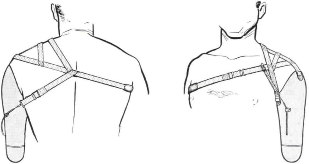
Fig. 19. The above-elbow chest-strap harness with webbing shoulder saddle. The functional arrangement is identical to that in the above-elbow chest-strap harness with leather shoulder saddle (Fig. 18). The leather has simply been replaced with a webbing saddle designed to give the same function. The technique is best used on individuals who perspire freely but who nevertheless need the chest-strap type of harness for heavy lifting.
