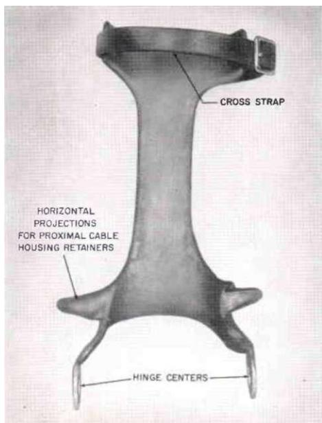
Fig. 9. Alternative design of the UCLA epicondyle cuff, constructed of stainless steel and covered with horsehide, the rigid hinges being attached to the cuff before covering. The cross strap at the top helps to stabilize the cuff on the arm.
