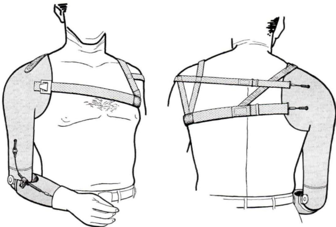
Fig. 23. Shoulder-disarticulation harness using scapular abduction for dual control, elbow lock being operated by flexion of the shoulder on the sound side. After Pursley (23), by permission of *Orthopedic and Prosthetic Appliance Journal*.
