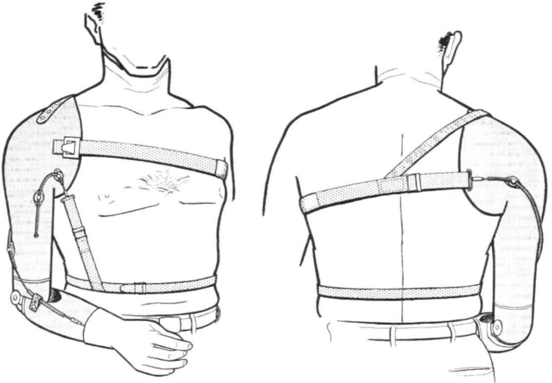
Fig. 22. Shoulder-disarticulation harness using scapular abduction for dual control, elbow lock being operated by shoulder elevation on the amputated side. After Pursley (23), by permission of *Orthopedic and Prosthetic Appliance Journal*.
