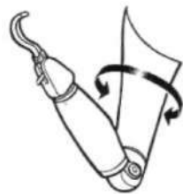
Fig. 7. Test for socket stability during arm rotation.
