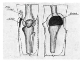
Fig. 33. The supracondylar-wedge suspension method.
