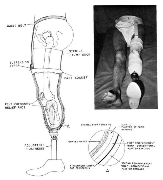
Fig. 18. Schematic cross section showing the major elements of a prosthesis as applied immediately following surgery to a below-knee amputee. The suture line, silk dressing, and drain are not shown. The fluffed gauze does not extend beyond the area indicated in "A." *Inset:* A below-knee amputee fitted with the immediate postsurgical prosthesis.
