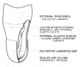
Fig. 34. Cutaway view of the air-cushion socket.
