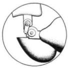
Fig. 12. Robin-Aids stump-actuated elbow lock.
