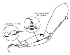
Fig. 16. Bowden-type control cable and attachments.
