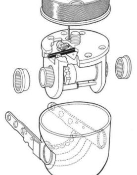
Fig. 13. Northrop model C elbow unit.
