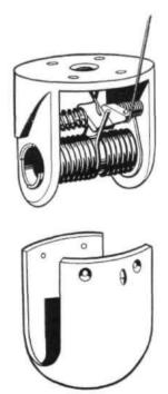
Fig. 14. Hosmer elbow unit, without turntable or forearm saddle attachments.
