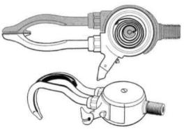
Fig. 4. Northrop-Sierra voluntary-opening two-load hook. Schematic diagram (above) shows arrangement of hook thumb and enclosed coil springs.
