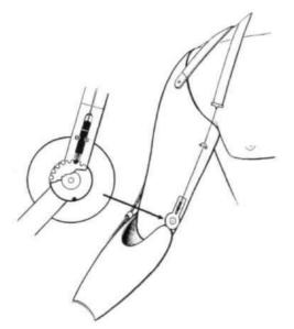
Fig. 15. APRL-Sierra outside-locking elbow hinge.
