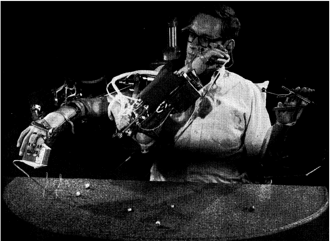
Fig. 7. The Case Research Arm Aid, Mark I. The pneumatic system shown allowed five degrees of freedom through the shoulder, arm, and wrist. Modifications being made include conversion from a pre-programmed tape control to computer-calculated trajectories by means of myoelectric input control signals.
