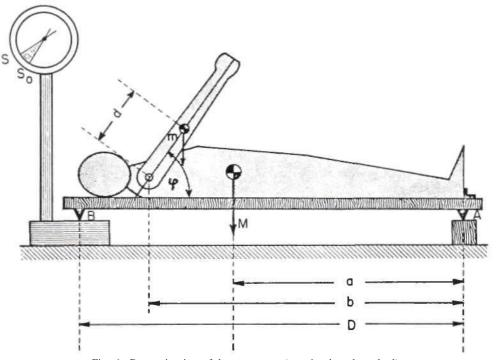
Fig. 6. Determination of the arm mass (reaction-board method).
