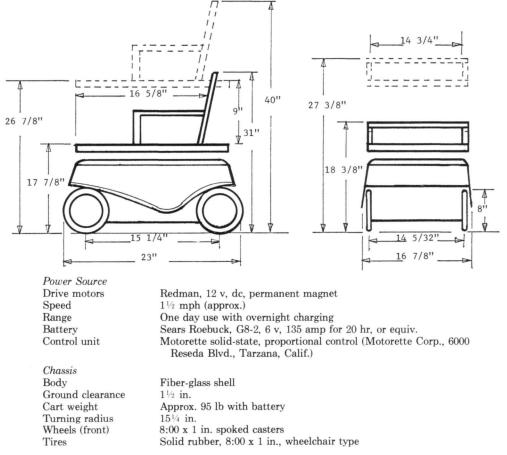
Fig. 6. Dimensions and specifications of CAPP electric cart.
