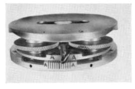
Fig. 4. The adjustable coupling assembled.
