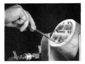
Fig. 8. Attaching the top assembly of the coupling to the bottom surface of the above-knee socket
