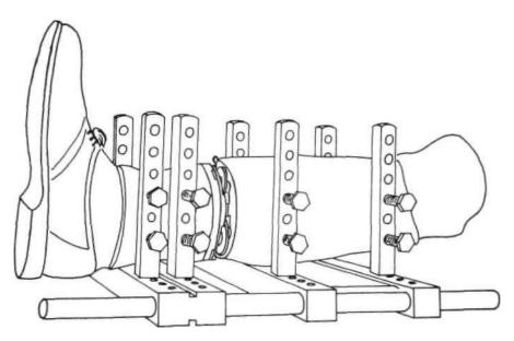
Fig. 14. Special band-saw jig used by Danes during alignment transfer. This jig holds components of the prosthesis in a fixed position to allow parallel band-saw cuts on both sides of the coupling. Subsequent clamping after cementing of wood block to replace coupling is also facilitated by this device.
