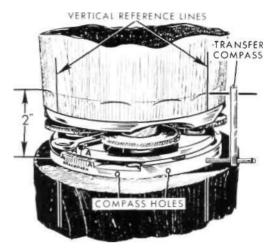
Fig 10. Use of the special compass for an alignmenttransfer reference. The vertical reference lines will be used to reestablish anteroposterior, mediolateral. and rotation positions. The horizontal line tangent to the tops of the compass arcs will reestablish tilt. From (10).
