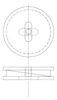
Fig. 19. Schematic drawing of the "Wilson-Riblett wedge," as applied to the VAPC coupling.
