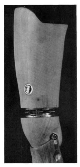
Fig. 6. The coupling installed in an above-knee prosthesis.
