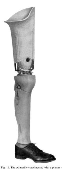
of-Paris above-knee temporary sockel and an unfinished knee shank. The three straps are each 1/8 in by 3/4 in. low-carbon steel. From (9).
