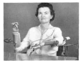
Fig. 9. Present-day Georgia Warm Springs Foundation feeder, the balanced forearm orthesis.
