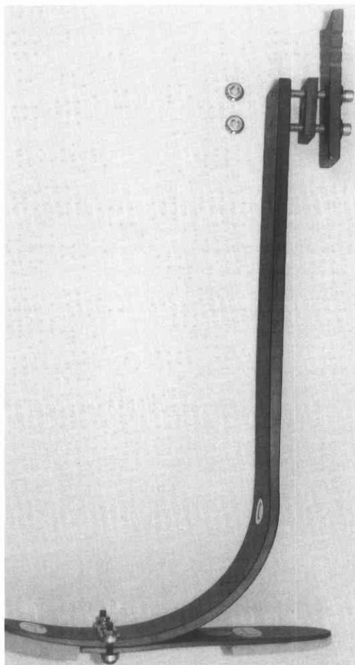
Figure 3. Modular Flex-Foot ™ (MFF), showing improved socket and heel attachment designs.
