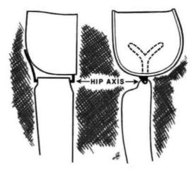
Fig. 5. Variations in tilting-table prostheses: hip joint below socket. Left, anterior view; right, medial view.
