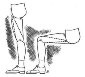
Fig. 11. Steps in the evolution of the Canadian-type hip-disarticulation prosthesis: floating thigh cover for cosmesis.
