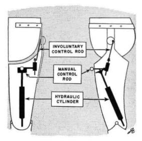
Fig. 7. Navy hydraulic prosthesis for hip disarticulation, schematic.
