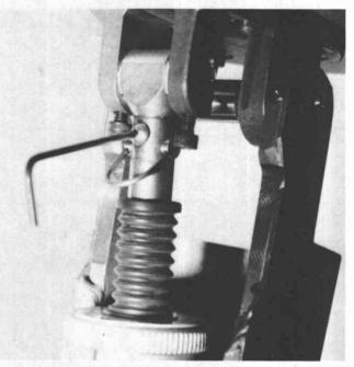
Figure 3. Allen wrench inserted into the stance adjustment screw.
