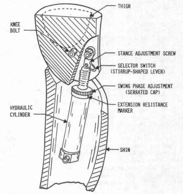
Figure 1. Cutaway diagram of the Mauch Unit
